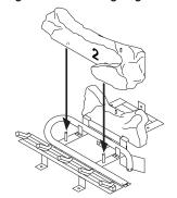
Figure 45 - Installing Log No. 2
